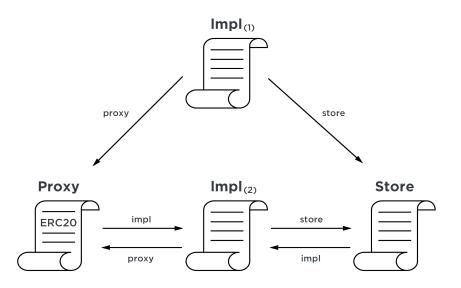
The above diagram reflects a post-upgrade state of the world, whereby the previous instance of 'Impl'(1) has been replaced by a new instance of 'Impl'(2). The instance of 'Proxy' now delegates to 'Impl'(2). Similarly, the instance of 'Store' now only accepts calls from 'Impl'(2). The previous instance of 'Impl' remains, but has become inert because it is now unlinked from the system.
